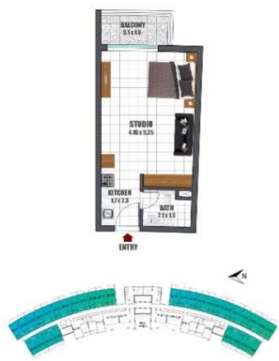
TYPICAL STUDIO UNIT FIRST FLOOR AREAS - 400.7 - 400.40 sq.m WING A - Flat Nos. - 03, 04, 05, 06, 07, 08, 09, 10, 11, 12, 13, 14, 15, 16, 17, 18 WING B - Flat Nos. - 03, 04, 05, 06, 07, 08, 09, 10, 11, 12, 13, 14, 15, 16, 17, 18
